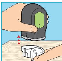
**Do not** detach the pedestal from the serter in mid-air, as this might damage the Enlite™ sensor.
